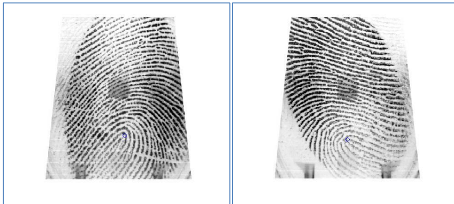
Figure (6.7): The results of detection the core point in left loop and right loop fingerprint image classes.
